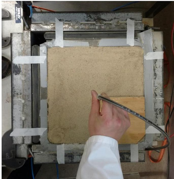
Fig.4.12. Horizontal centralization of the pressuremeter probe
