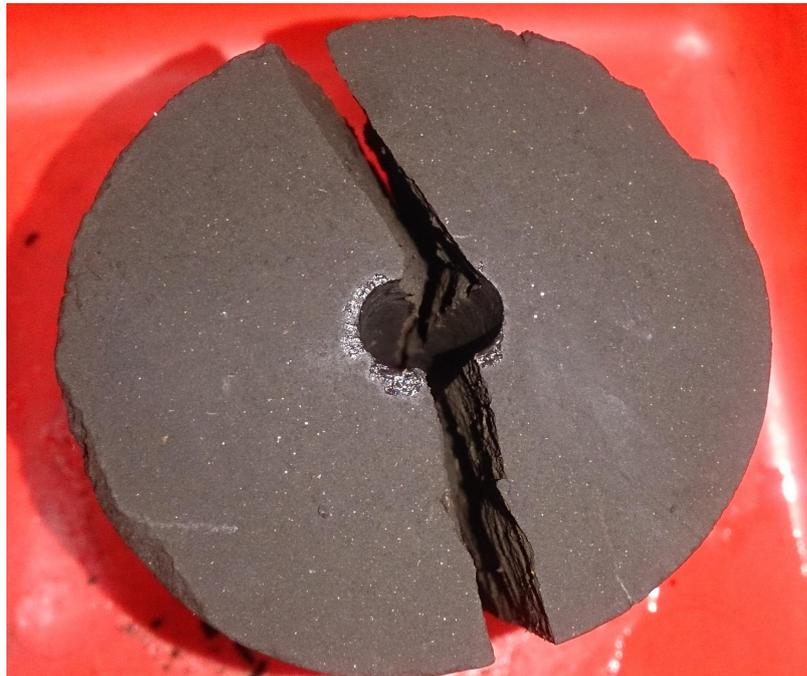
Fig.4.42. Brown coal UET specimen after the secondary failure
