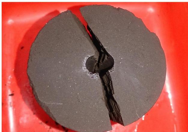
Fig. 10. Brown coal UET specimen after the secondary failure.
