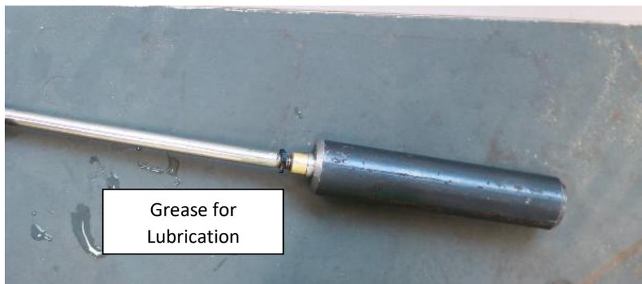
Fig.4.7. Inserting probe into calibration hose
