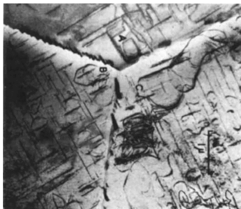
Fig. 2.21 Three boundaries with misorientations of 4^\circ (AB), 6^\circ (BC) and 9.5^\circ (AC) in an Al-4Cu alloy after 2 h ageing at 240^\circ \text{C} . Boundaries AB and BC contain \theta' precipitates, boundary AC contains \theta precipitates. Reproduced with permission from [109].
