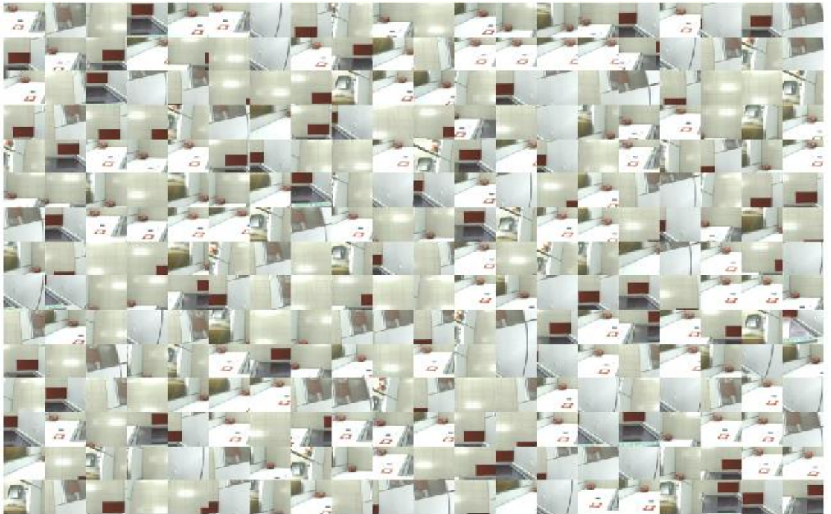
Figure 5.6: Examples of a) pedestrian instances and b) non-pedestrian instances autonomously acquired and labelled by VAT, from Site 1, during scene-specific training of the overhead-pedestrian detector.
