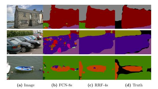
Figure 5.4: RRF-4s results on MSRC-21 Test data: Column (b) shows the segmentations produced by the baseline CNN model [135]. The output of our highest performing model, RRF-4s, is shown in column (c). Comparatively, our system seems to be more robust at detecting changes in texture (first row), handles occlusion better (second row) and better handles irregular lighting conditions (third row).
