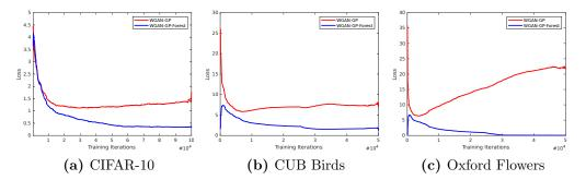
Figure 7.10: Critic loss curves for WGAN-GP and WGAN-GP-Forest over (a) 100k training iterations for CIFAR-10 (b) 50k training iterations for CUB Birds and (c) 50k training iterations for Oxford Flowers. Across all 3 datasets, we note that the critic loss for our WGAF-GP model shows better critic loss convergence over the WGAN-GP baseline.
