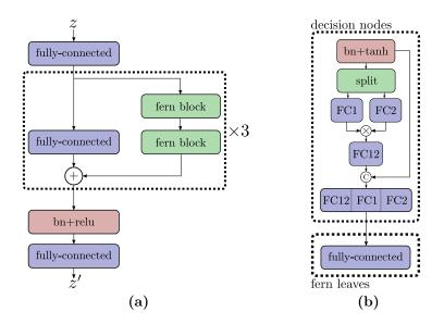
**Figure 8.5:** (a) The architecture of our proposed transformer network. (b) The structure of a fern block used in our transformer network. We use a reparameterisation trick which allows for the construction of soft decision ferns using common network components such as FC linear layers and Hyperbolic Tangent activation layers.
