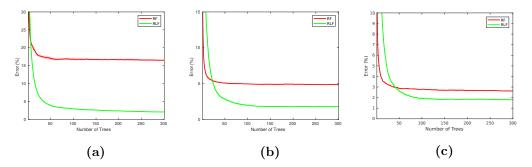
**Figure 4.1:** Classification error of RLF vs. RFs varying the number of trees from [1, 300] for a fixed maximum tree depth of (a) 5, (b) 10 and (c) 15 on the *MNIST* test data. For shallower trees, our RLFs significantly outperforms RFs. In each case, we report mean result across 10 separate runs.
