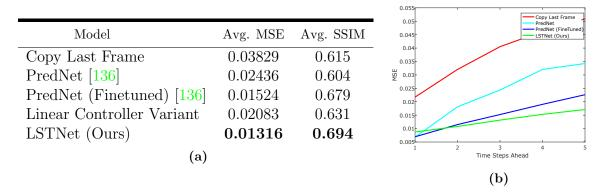
Figure 8.7: (a) Averaged MSE and SSIM over 5 timesteps of frame prediction (b) Individual MSE for each predicted time step plotted for Copy Last Frame, PredNet and LSTNet.
