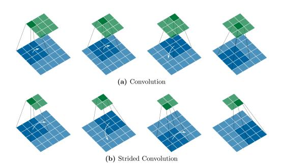
**Figure 3.11:** (a) A 2D convolution layer operating on the input with a stride of 1 and a kernel size of  $3 \times 3$ . In this case, each pixel is densely sampled and the output is not downsampled (reduction in size of the output is due to the size of the kernel). (b) A strided 2D convolution layer with  $3 \times 3$  kernel size and stride of 2. Due to the increased stride, the spatial size of output is downsampled from the spatial size of the input.
