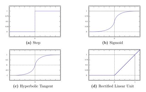
Figure 3.9: Commonly used activation functions employed in deep neural networks. Each activation function serves to break the linearity that exists between successive convolution or fully connected layers in a network, allowing them to model complex non-linear functions.
