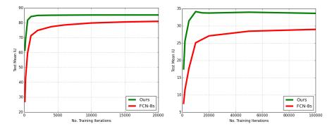
Figure 6.5: Training iteration timings vs. mean IU performance on KITTI (left) and NYUv2 (right) test data. The mean result across 10 separate runs is shown.
