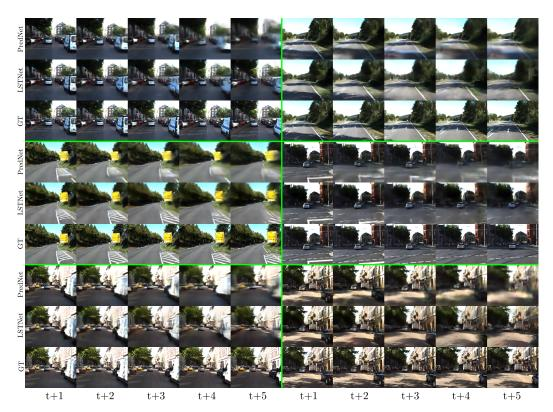
**Figure 8.9:** Multi-Frame predictions. This figure depicts of 6 sequences selected from the KITTI test set where  $\{I_{t+1}, I_{t+2}, I_{t+3}, I_{t+4}, I_{t+5}\}$  are predicted using a past sequence of 5 frames. Each example is organised into 3 rows depicting PredNet (FineTuned) [136], our LSTNet and the ground-truth for comparison.
