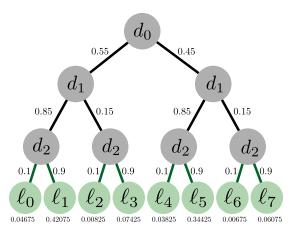
**Figure 8.4:** A decision fern with soft routing. Each decision node determines a routing portion to subsequent child nodes. The decision nodes along a route determine the final routing portion to all terminating leaf nodes, instead of the hard route approach which selects a single path to a single leaf node.
