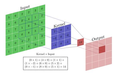
Figure 3.7: A convolution operation on an image patch. The kernel is operated on a sliding window across the entire input image where it is convolved with patches in the input image. The result of each convolution of an image patch with the kernel results in an output pixel value as shown.
