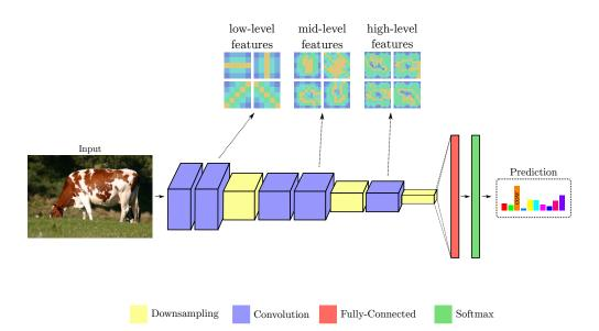
Figure 3.6: A common CNN architecture used for image classification consisting of convolution and downsampling layers, followed by a fully connected linear layer and Softmax [9] layer. As shown, features extracted by filters earlier in the CNN architecture are simpler, extracting points and edges. These earlier layers build up to more complex features in deeper convolution layers in the CNN to detect more complex shapes.
