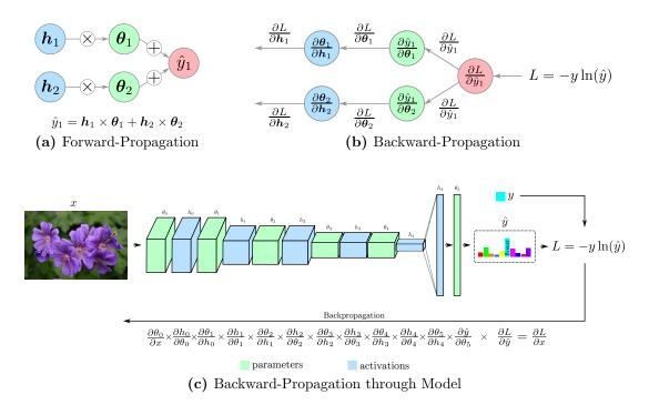
Figure 3.13: (a) Forward propagation on the last part of a neural network. Input activations  $h_i$  are propagated through and multiplied with the parameters of the network  $\theta_i$ . (b) Backward propagation propagates derivatives back through the network to the corresponding parameters in the network via use of the chain-rule. (c) Backward propagation through a model for an image classification task. Gradients are computed via the chain rule.
