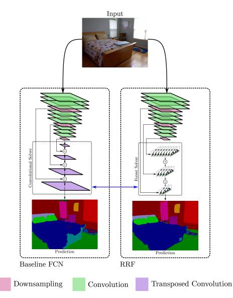
**Figure 5.1:** Our RRF model replaces the fully convolutional solver component of a baseline FCN. Instead of using skip connections to the activations of earlier convolution layers in the network, we build a decision forest directly from the activations of specified convolution layers in the CNN.
