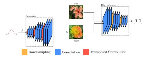
Figure 7.1: A typical generator/discriminator setup in the original formulation of the GAN. The generator's role is to generate fake images from a source of energy (typically Gaussian or uniform distribution) that can fool the discriminator, whose role is to distinguish between real and fake images. Correct training between these two adversaries results in an equilibrium state where they are evenly matched
