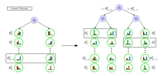
Figure 3.4: The ID3 algorithm selects a decision function based on an entropy minimising criteria. A decision tree is recursively constructed in this manner.
