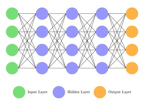
Figure 3.5: A typical feed-forward network architecture. The network consists of stacked fully-connected linear layers (non-linear activations are not shown). Each neuron of each layer is connected to all neurons in the proceeding layer.
