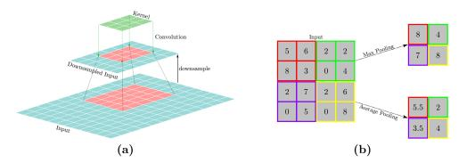
**Figure 3.10:** (a) For a  $3 \times 3$  kernel operating on a downsampled input, the effective receptive field the kernel has on the original input is increased to  $5 \times 5$ . In this way, downsampling layers allow smaller kernels to capture more context of the surrounding area around a given centre point. (b) Two common downsampling operations, max pooling and average pooling.
