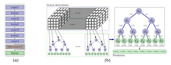
Figure 7.5: An overview of our proposed changes. (a) shows our architecture which modifies the discriminator/critic network by replacing its fully-connected layer with a decision forest (Batch Normalisation/Layer Normalisation is not shown). (b) shows reshaping of conv4 activations in DCGAN/WGAN-GP to form our decision node parameters.
