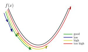
**Figure 3.14:** When the learning rate is too high (red) or too low (blue), the model either fails to converge to a solution or converges very poorly. Setting a relatively high learning rate (yellow) may lead to short term gains in performance but this can quickly saturate as the model approaches the local minima and begins to overshoot it. A good learning rate (green) should be able to learn quickly but should not miss any local minima it can converge towards.
