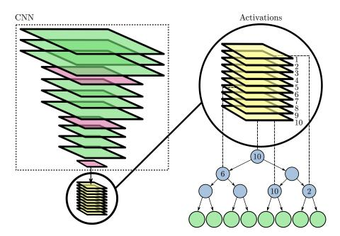
**Figure 6.1:** Each decision node is initialised by being randomly assigned a channel index from the feature activation map of its corresponding convolution layer. The decision function in each decision node consists of a channel index value which indexes into a channel of the input feature map to obtain an activation value. This is then compared with the decision node's assigned threshold value to determine routing direction.
