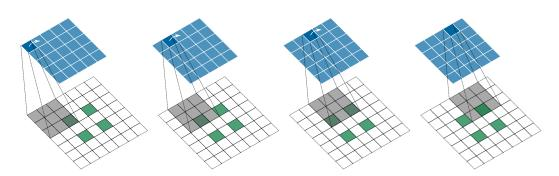
Figure 3.12: A transposed 2D convolution with stride size of 2, kernel size of 3 and no padding. This operation produces a  $5 \times 5$  output with a  $2 \times 2$  input.
