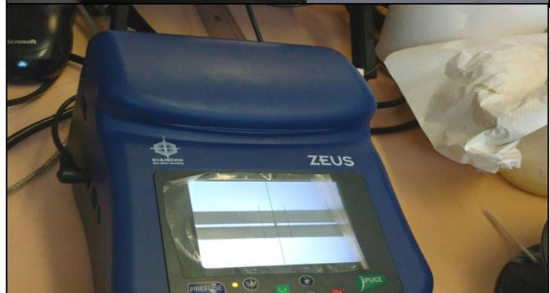
Figure 7.4 Steps for splicing and fusing optical fiber
