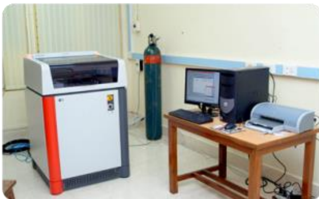
Figure A3.1 Figure X-ray fluorescence spectrometer used in the study at IIT Bombay
