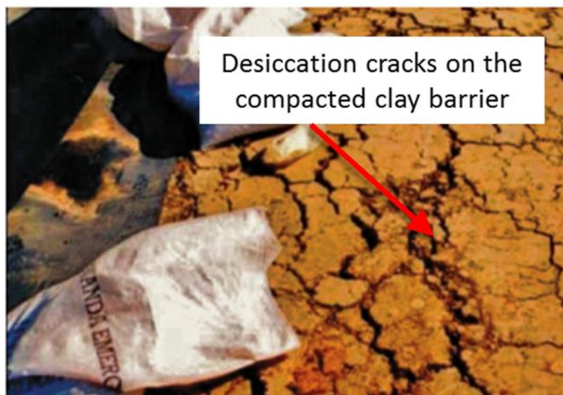
Figure 2.6 Compacted clay liner (forming part of a composite liner) that has desiccated (After Rowe, 2012)
