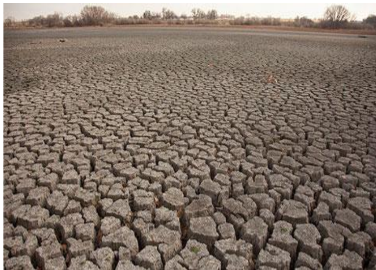
Figure 1.8 Desiccation cracking in soils in drought affected Vidarbha, India (Source: https://indianexpress.com/article/india/india-news-india/marathwada-dams-to-be-interlinked-water-grid-proposed-for-effective-management-2855513/ )
