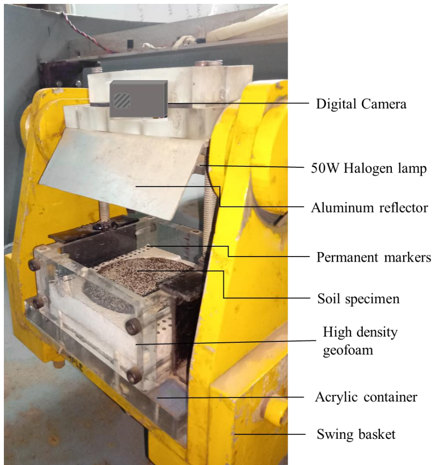
Figure 8.4 Perspective view of the test setup mounted onto swing basket of the centrifuge
