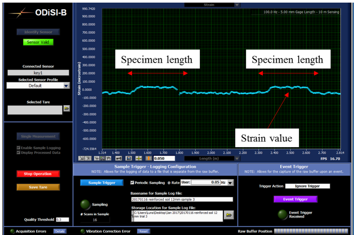
Figure 7.10 ODiSI-B Sensor Configuration Graph Screen when compressive strain is developed in the soil
