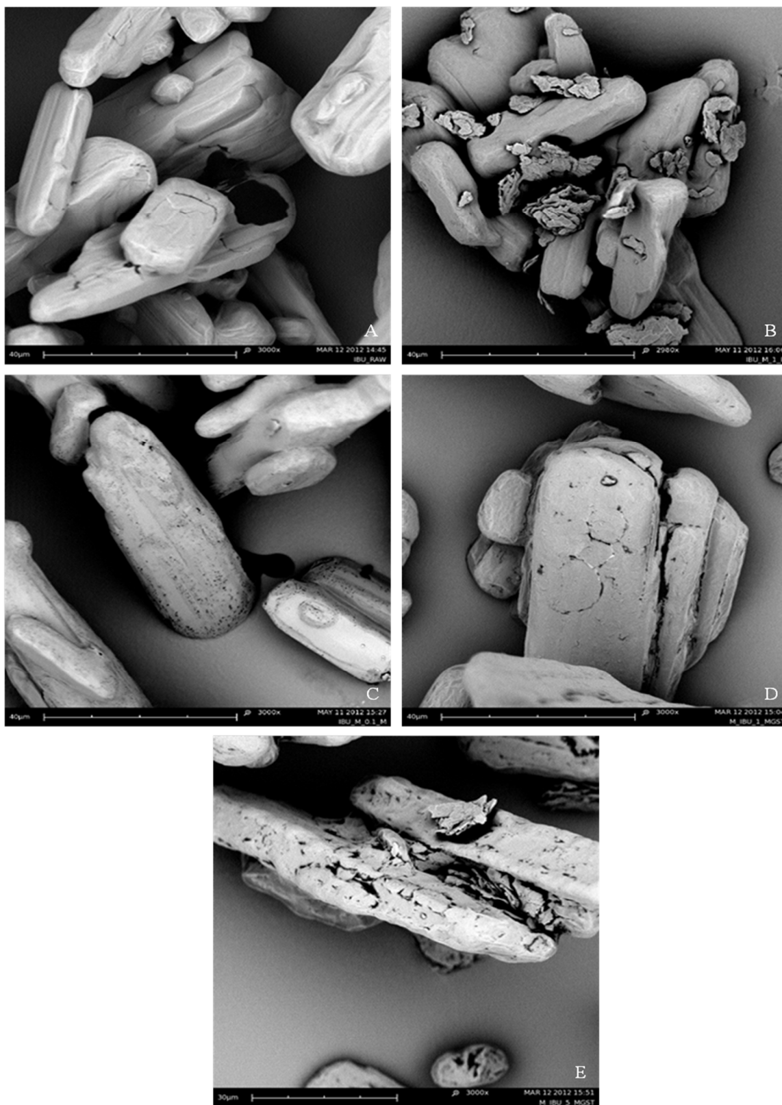
Figure 4. SEM micrographs of ibuprofen samples at magnification of 3000 \times (A: raw particles; B: MgSt-blended particles; C: 0.1%MgSt-mechanofused particles; D: 1%MgSt-mechanofused particles; E: 5%MgSt-mechanofused particles), scale bar represents 40 \mu m in micrograph of A, B, C, D and 30 \mu m in E.
