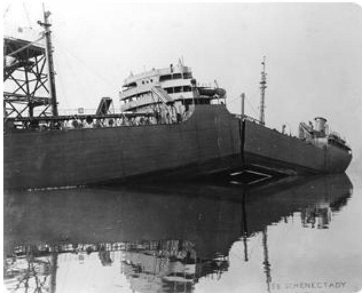
Fig. 2.1 Failure of the Liberty ship due to a crack initiated at the weld ( http://www-g.eng.cam.ac.uk/125/1925-1950/tipper3 ).
