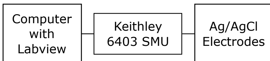
Figure 3.5: The basic setup for conducting ion current measurements in a sensitive system
