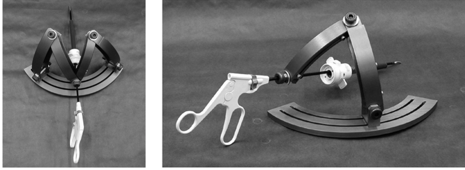
Figure 2.11: Sample serial spherical linkages (right) and its parallel (left) configuration [123].
