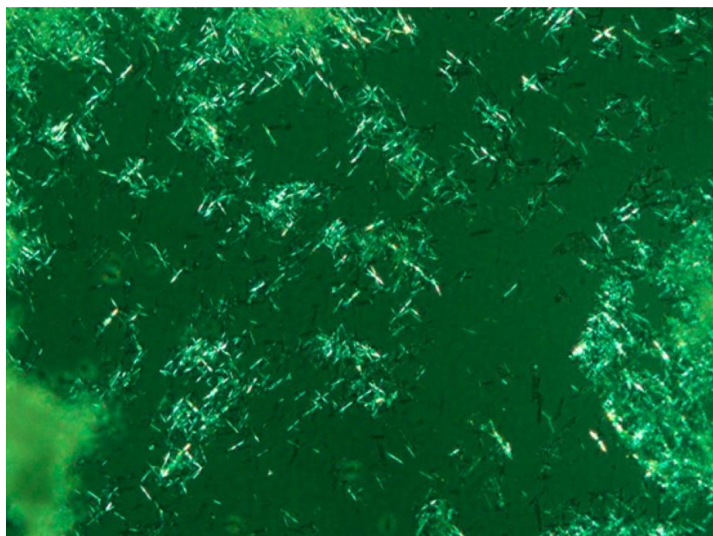
Figure 4: Crossed polarized light microscopy image of the pellet phase obtained from the lipolysis experiment at pH 8.0. Crystalline cinnarizine was observed as many needle-like structures.
