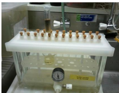
Figure 2.2 Pressure manifold utilised to carry out protein purification.
