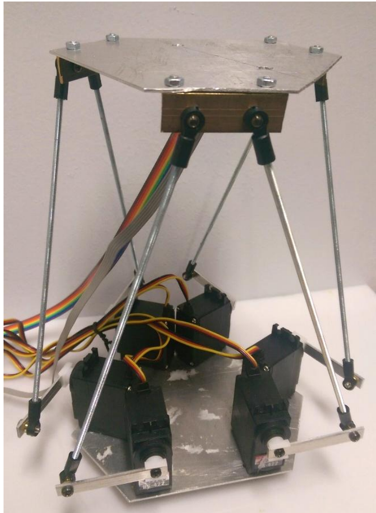
Figure 7 – 6-DoF Stewart platform arrangement with 6 servomotors
