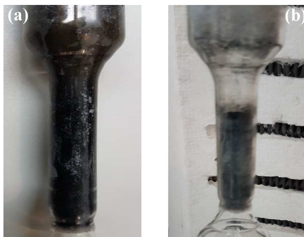
Figure 5.22: Guaiacol conversion a) without a catalyst and b) in the presence of catalyst
