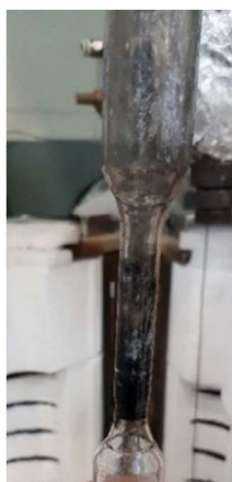
Figure 5.17: Picture of the reactor after reaction: T=500°C, 0.5 g of Rh-Ni/ \gamma -Al 2 O 3 , C/O=1.3, and S/C=0
