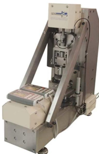
Figure 3.5 GDS Standard Simple Shear System (GDS-STDSS)
