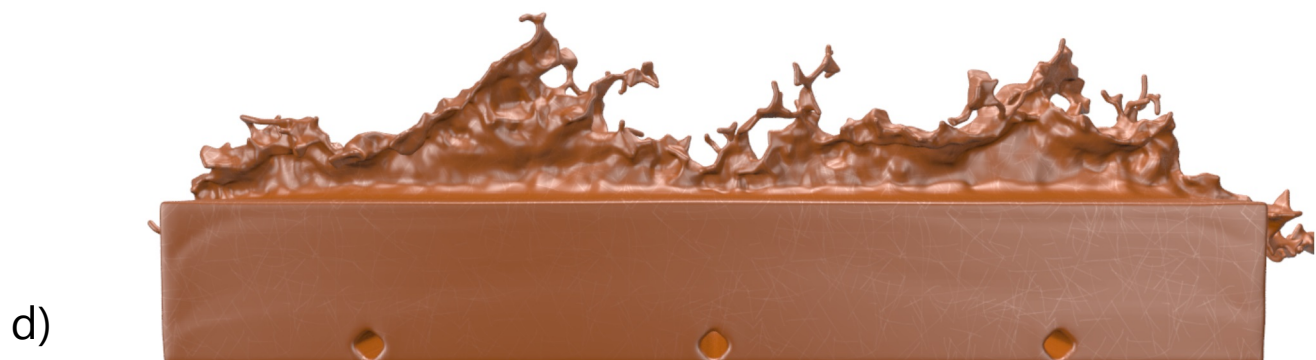
Figure 5.20: Copper flashing after processing (experimental and numerical) shown by a) Advancing side - Experiment (processing direction to the left), b) Advancing Side - Numerical, and c) Retreating side - Experiment (processing direction to the right), d) Retreating side - Numerical. Note that the thermocouple holes were machined on the other side to the simulation for this particular plate.
