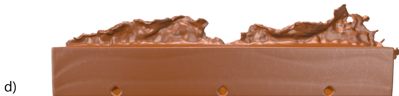
Figure 6.23: Copper flashing after processing (experimental and numerical) shown by a) Advancing side - Experiment (processing direction to the left), b) Advancing Side - Numerical, and c) Retreating side - Experiment (processing direction to the right), d) Retreating side - Numerical. Note that the thermocouple holes were machined on the other side to the simulation for this particular plate.
