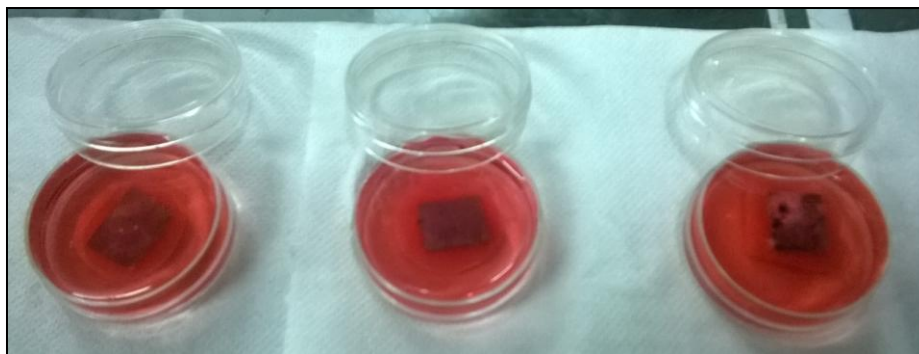
Figure 3.5: Mounted magnesium alloy samples immersed in DMEM in petridish
