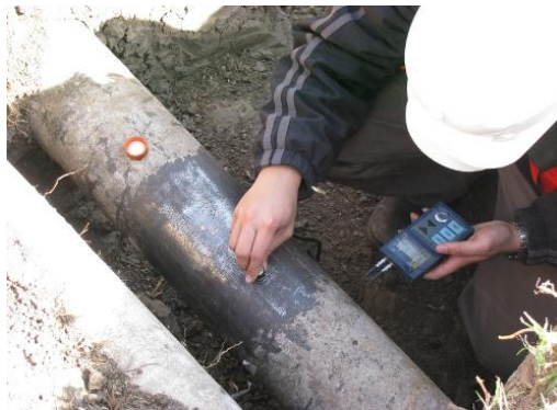
Figure 3-30 Measurement of water pipe wall thickness with ultrasonic gauge
