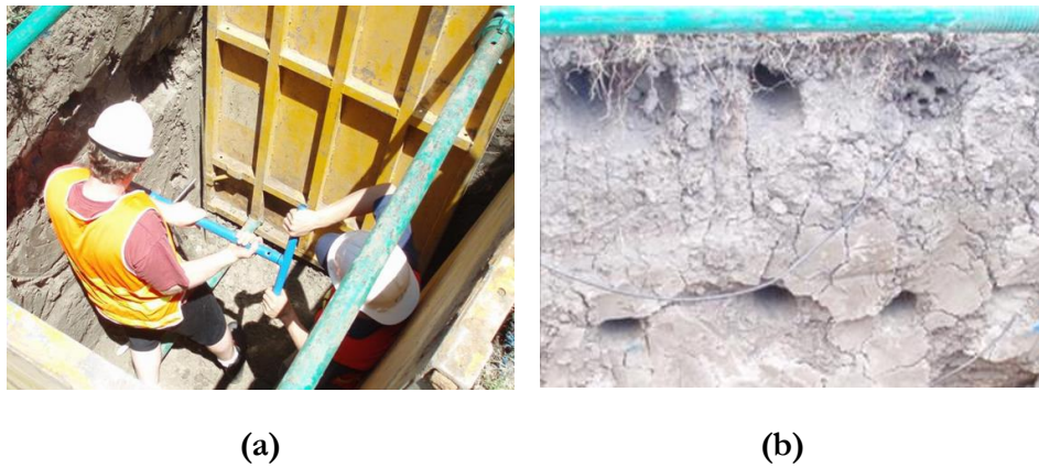
Figure 3-35 Preparation of horizontal holes: (a) drilling with hand auger; (b) a view of the drilled holes
