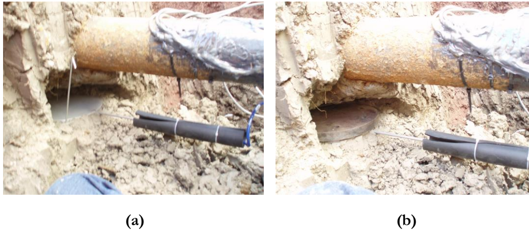
Figure 3-33 Earth pressure cell installation: (a) placed beneath water pipe; (b) with steel plate placed on top
