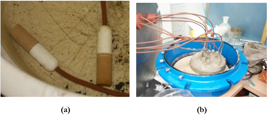
Figure 3-13 Thermal conductivity sensors: (a) in saturation; (b) in a pressure plate for calibration
