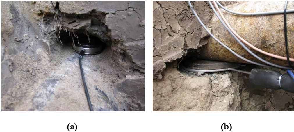
Figure 3-52 Earth pressure cell: (a) a micro-strain type installed above the pipe; (b) a vibrating wire type installed beneath the pipe
