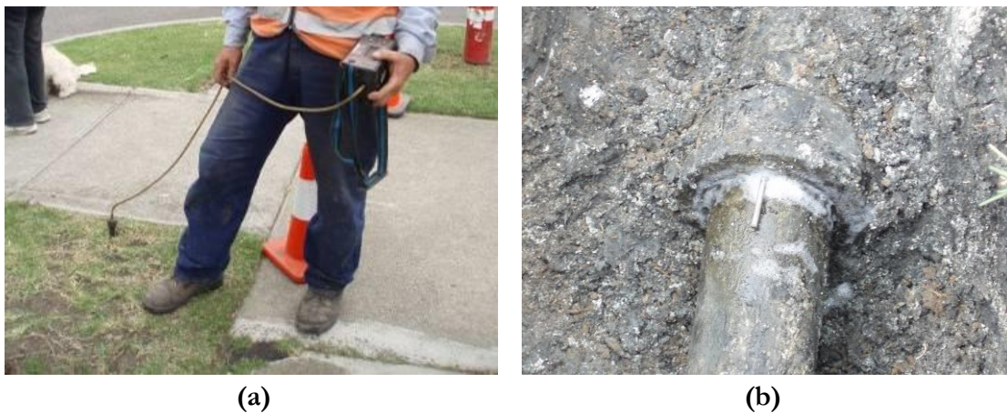
Figure 3-3 Detection of gas pipe leaks with gas emission sensor: (a) A gas emission sensor inserted into the ground close to the suspected leak location; (b) Detergent sprayed on the failed pipe joint
