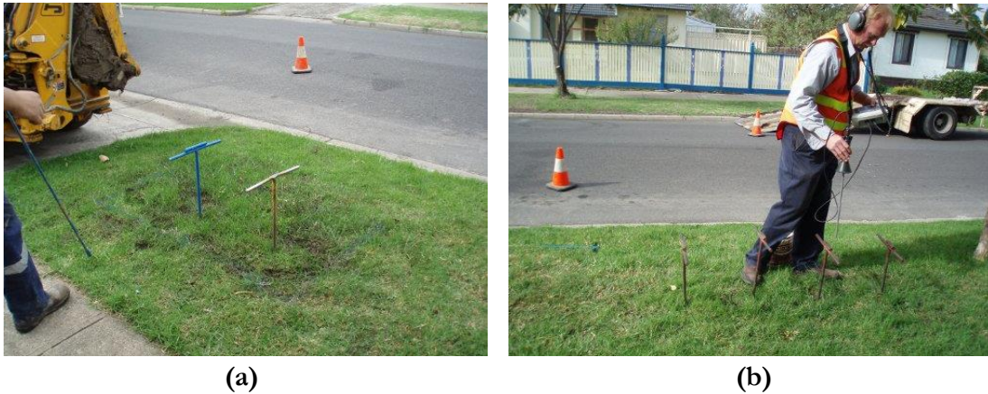
Figure 3-1 Detection of water pipe leaks by acoustic method: (a) Steel “T” bars placed along suspected pipe leak location; (b) “Listening” to the acoustic noise of water pipe leaks
