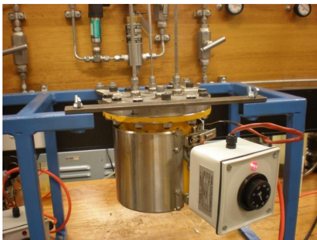
Figure 4.5: Image of supercritical CO 2 high pressure autoclave setup, with stainless steel lid closed and thermal sleeve attached
