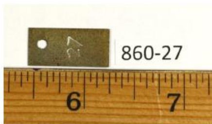
Figure B.9: Steel sample following exposure to 50000ppm water in a supercritical CO 2 environment for a period of 7 days
