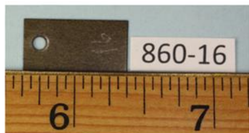
Figure B.7: Steel sample following exposure to 6000ppm water in a supercritical CO 2 environment for a period of 7 days
