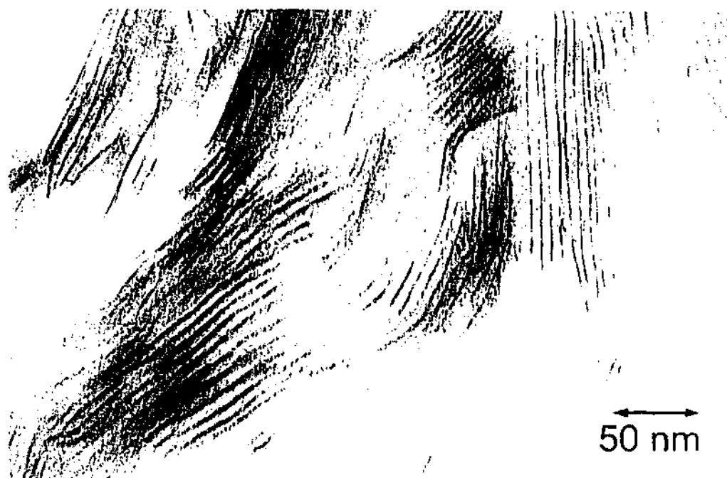
Figure 4.14: TEM micrograph of TGDDM nanocomposite cured at 100 °C (top) cured at 160 °C (bottom).
