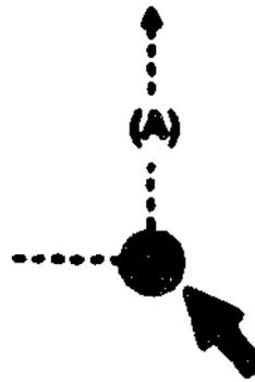
Figure 37: The direction of the net force on an object which turns  $90^\circ$
