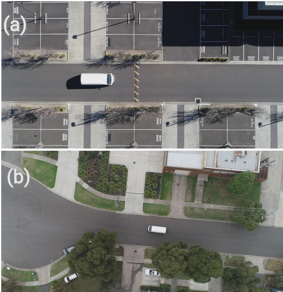
Figure 5-3: Aerial images recorded with the drone of the test vehicle (a) negotiating a speed bump, and (b) experiencing a disruption.
