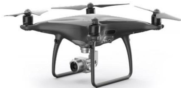
Figure 5-2: The Quadcopter, DJI Phantom 4 Pro used to obtain aerial video recordings of vehicle movement [147].
