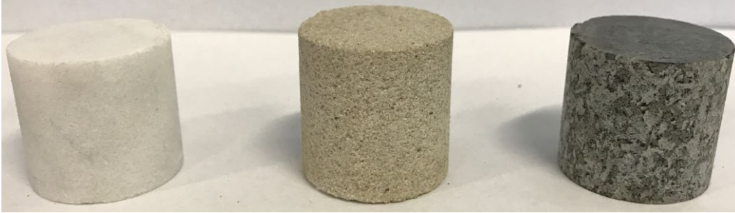
Fig. 3.2 Photograph of marble, sandstone and gabbro
