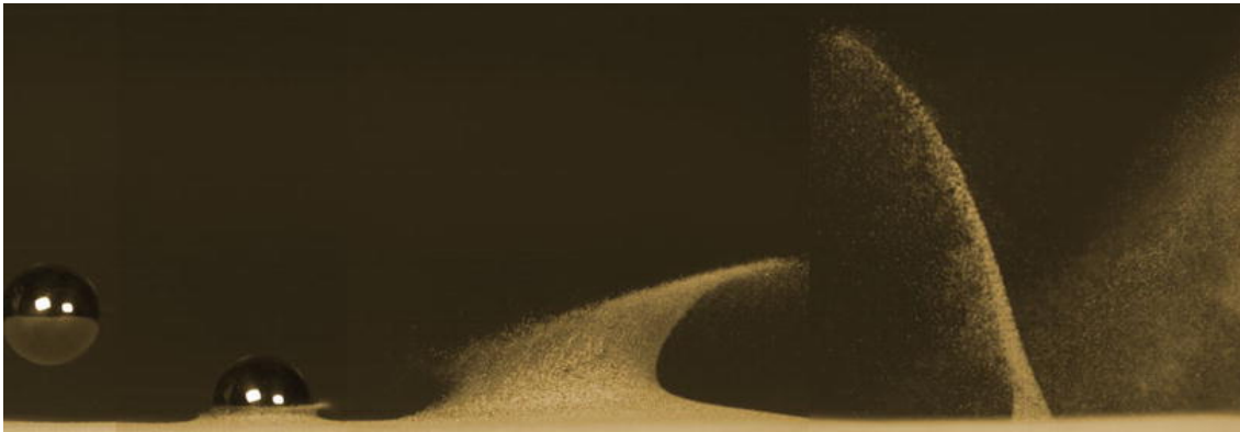
Fig. 3.17 An oblique impact of a steel ball into fine very loose sand creates a splash followed by a jet in the backward direction (Lohse, Bergmann et al. 2004).
