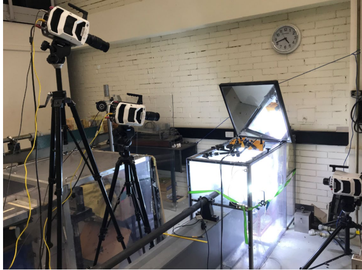
Fig. 6.4 Setup of three high-speed cameras in projectile impact
