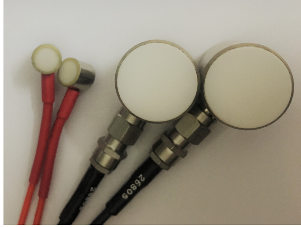
Figure 3.5: CTs of type Nano 30 and WD\alpha (MISTRAS Group) that are used in GW testing.
