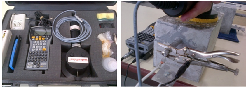
Figure 2.5: Galvanostatic pulse equipments used to test the corrosion of concrete specimens. Source: El-Dieb and El-Maaddawy, 2018.
